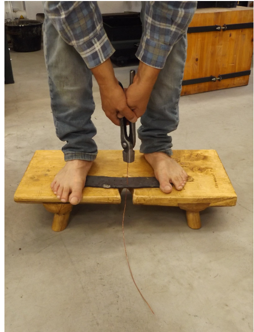
Abb. 4: Gezogener Kupferdraht (rund) am Ziehschemel. – Drawn copper wire (round diameter) at the foot stol.
