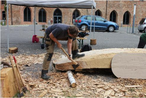
Abb. 5: Grobe Arbeiten am Heck. – Heavy works at the rear.
