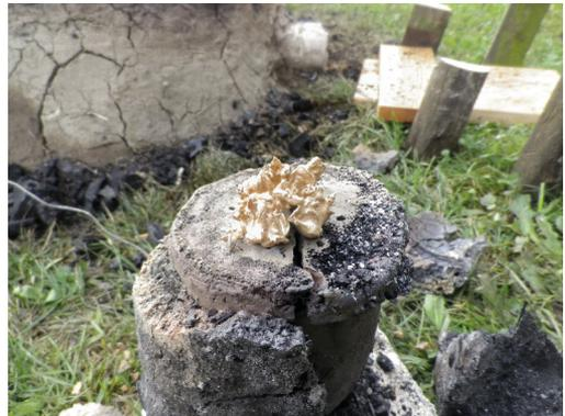
Abb. 5: Versuch 2, produziertes goldfarbenedes Messing. – Experiment 2, produced golden brass.
