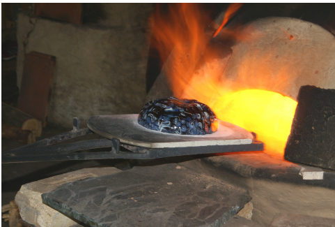
Abb. 6: Nachheizen einer Mosaikglas-Rippenschale. – Re-heating a mosaic ribbed bowl.
