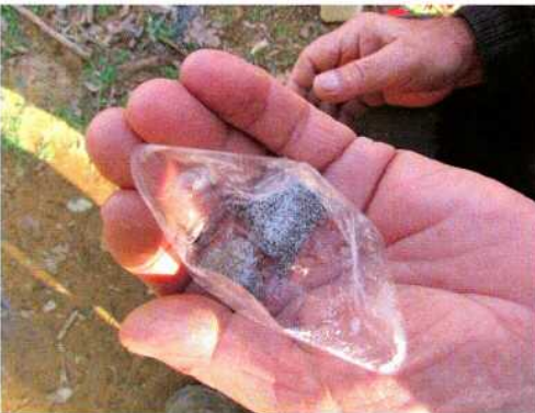
Fig. 7: Adding a flux (borax) to the gold concentrate. – Hinzufügen eines Flussmittels (Borax) zum Goldkonzentrat.
