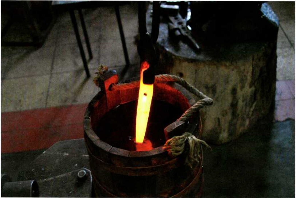
Abb. 8: Härten des Spitzenbereichs in Wasserbad. – Curing of the point in a water bath.
